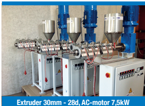
Extruder 30mm - 28d, AC-motor 7,5kW
