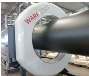
iNOEX WARP 1200 measuring system on Shengbang's PE pipe extrusion line
