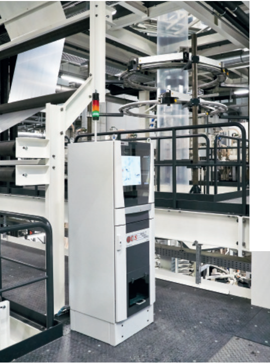
OCS Web Inspection System (FSP600) – Process integrated control unit
