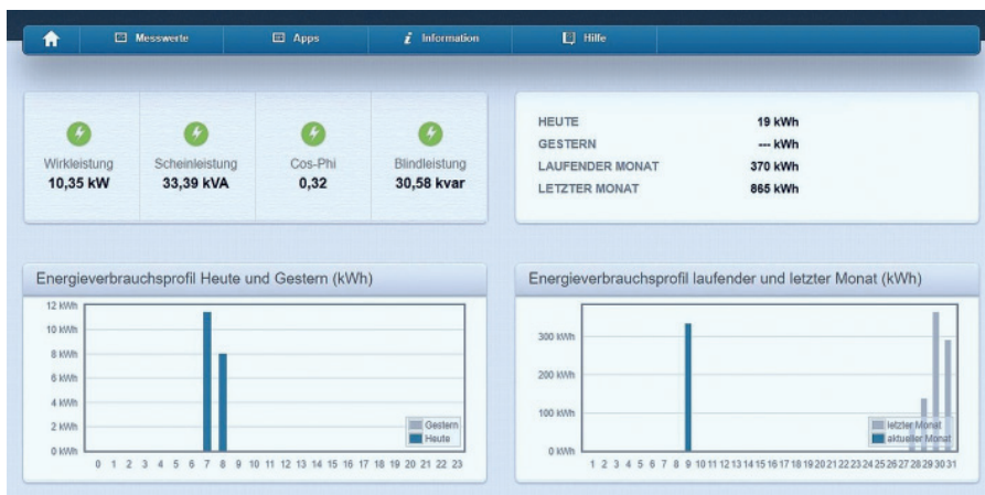
Getecha's energy consumption tool enables efficiency monitoring and performance optimisation of grinding plants (All images: Getecha)
