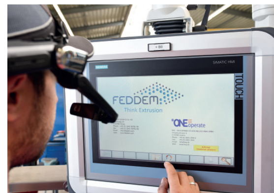
Direct operator guidance by means of data glasses via augmented reality projections
