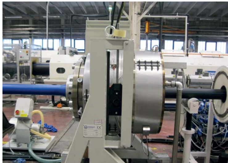
Co-extrusion of HSCR PE100 using a coating die head on a standard PE100 pipe
