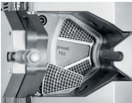
Filter disc and filter elements of the fully automatic Rotary Filtration System RSFgenius
