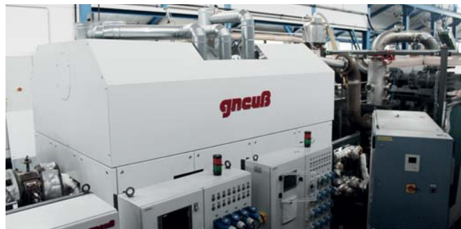
Polyreactor JUMP for flexible IV increase and adjustment
