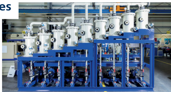
For a U.S. customer, BHS-Sonthofen designed a separation solution with a cascade wash. The separators have a stepped design
