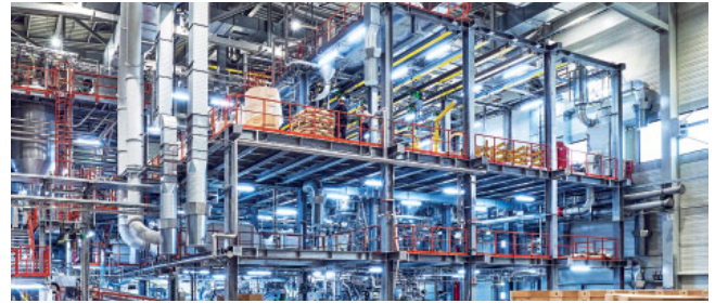
On its Coperion compounding system, LANXESS produces highly reinforced polyamide compounds at very high throughput rates (Photo: LANXESS, Krefeld-Uerdingen, Germany)
