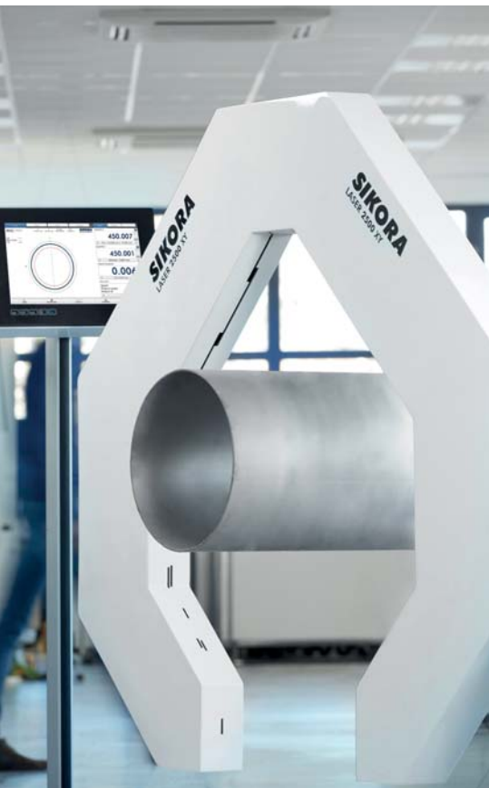
On the basis of laser technology, the LASER 2500 XY measures the diameter of wire rods, metal bars and tubes
