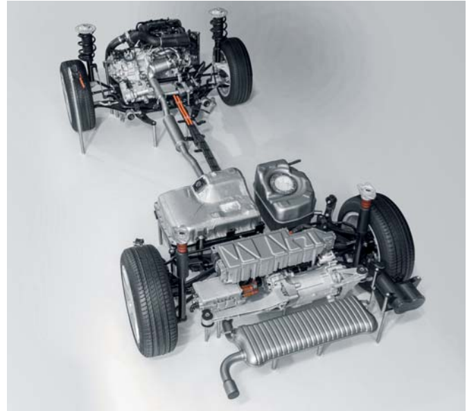
A look at the powertrain of the BMW 225xe. The electric motor of the plug-in hybrid vehicle BMW 225xe iPerformance won the Bavarian State Prize for E-Mobility (Photo: BMW Group)
