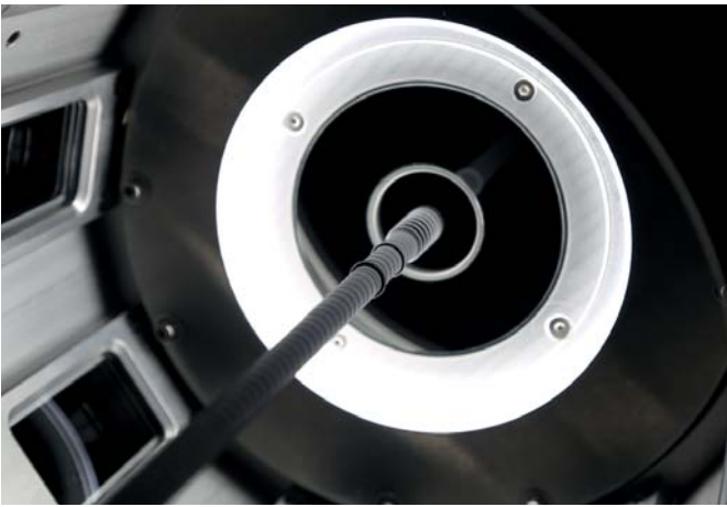
Entirely new algorithmic processes were developed for the surface inspection of corrugated tubing. Implemented in the inspection software, these algorithms now allow the recognition of the change from plane to wavy, and vice versa, and the masking out of different product structures
