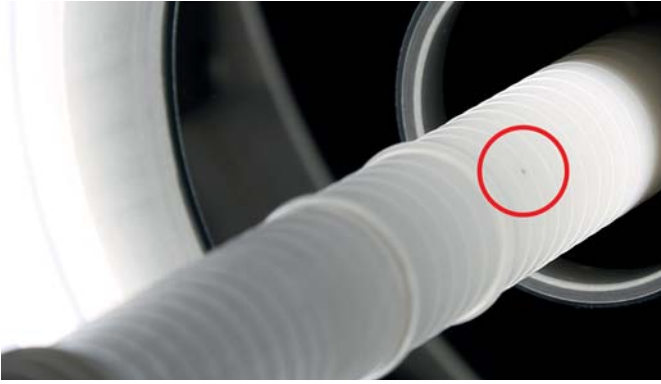
Also extremely small flaws, like the above shown tiny dent in a protective tubing for electronic wiring in cars, may easily become safety-critical. ProfilControl 7 S CorrugatedTube guarantees 100-percent quality of tubes for automotive engineering and many other demanding applications
