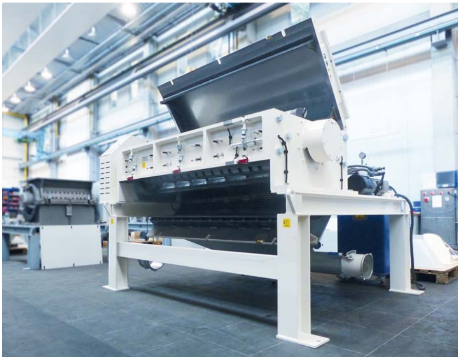
Universal granulator for recycling plastic waste – the Compact-Line from Hosokawa Alpine
