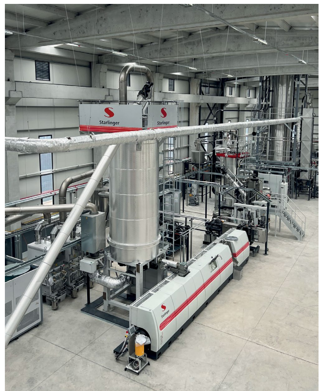
Starlinger's recoSTAR PET 165 HC iV+ recycling line will produce bottle-grade rPET pellets for Akmert's new brand "GSR GRANULES"
