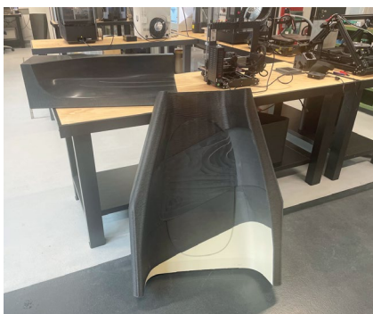
3D-printed laminating molds made with LUVOCOM 3F
