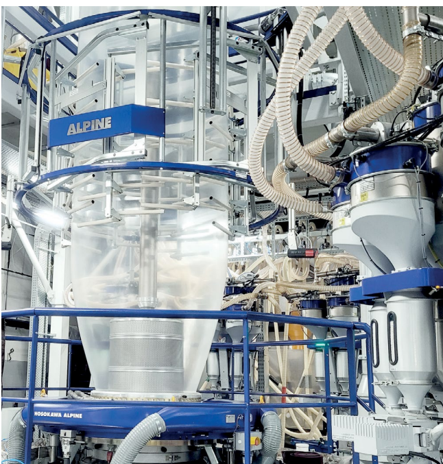
The new 7-layer line with inline MDO (Machine Direction Orientation) from Hosokawa Alpine at ERG in Poland
