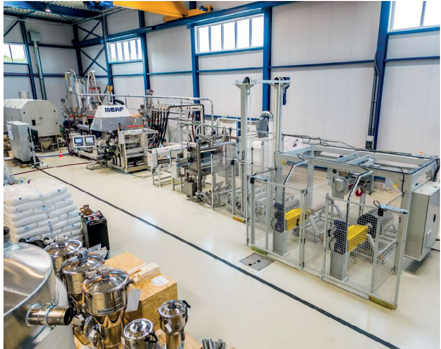
MEAF Machines has recently installed a first R-PET extrusion line for the production of meat packaging at Pack Klaipėda UAB in Klaipėda, Lithuania (Source: MEAF)
